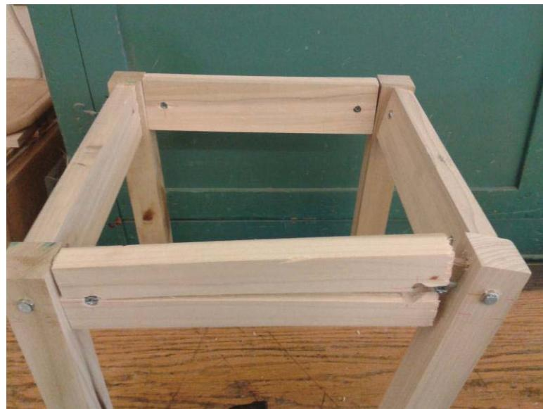
Failure on the stools with pinned round mortise and tenon joints.
