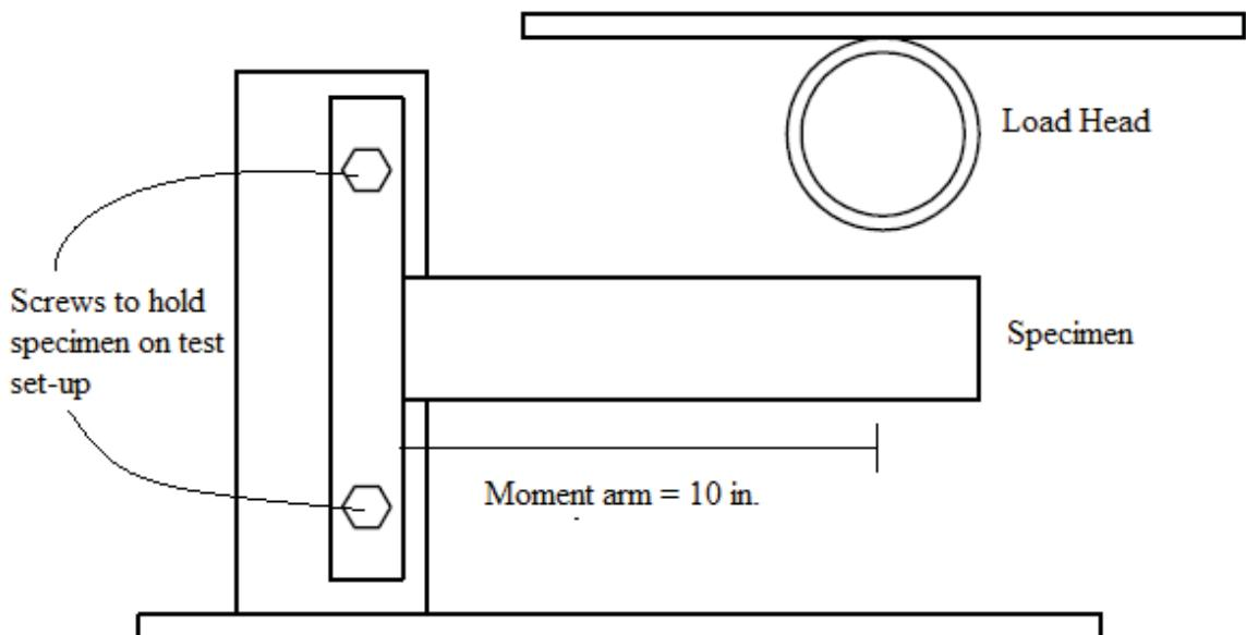
Figure 3-21: Static load test set up.
