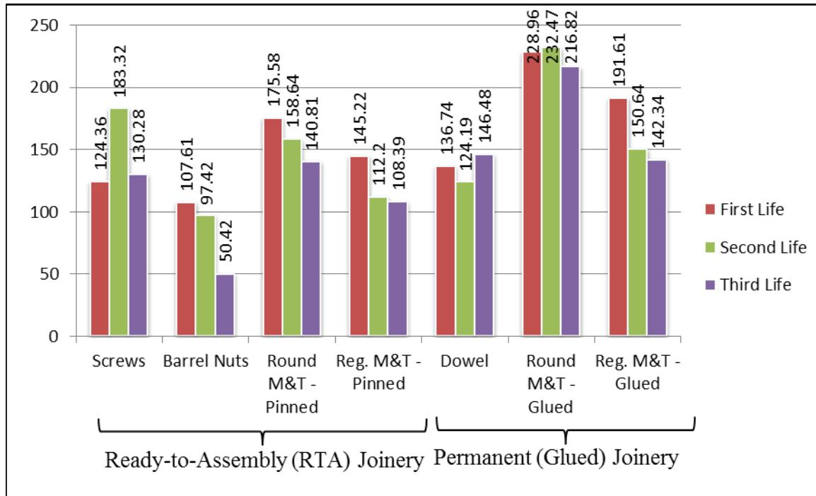
Figure 3-23: Average load carrying capacity of the stools with different joinery systems in each life.
