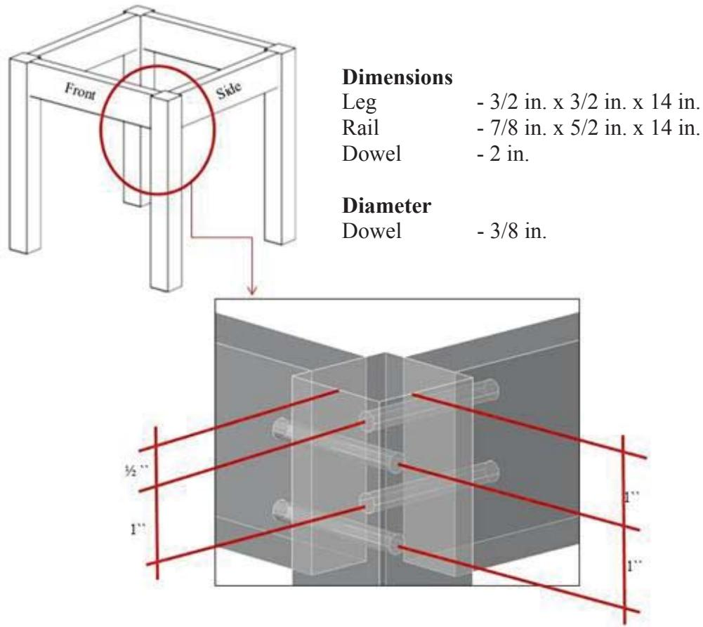
Figure 3-11: Dowel joint frame construction configuration
