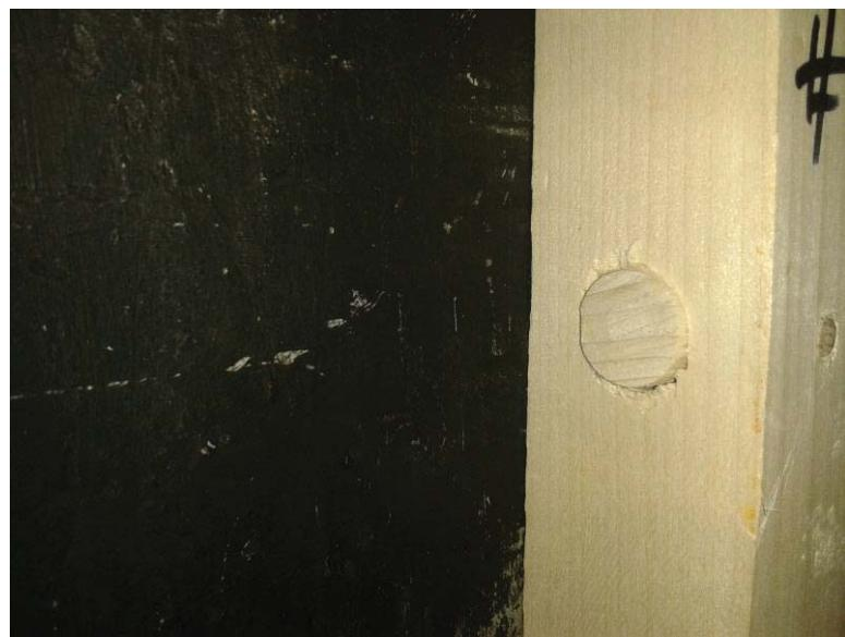
Failure on the L-shaped pinned rectangular mortise and tenon joints
