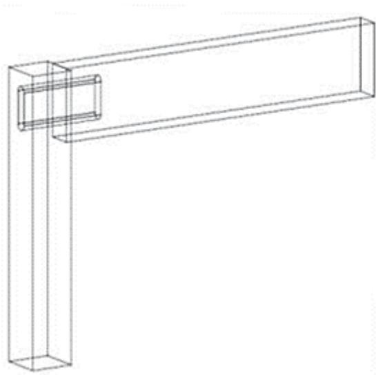
Figure 3-19: Glued rectangle mortise and tenon L-joint configuration.
