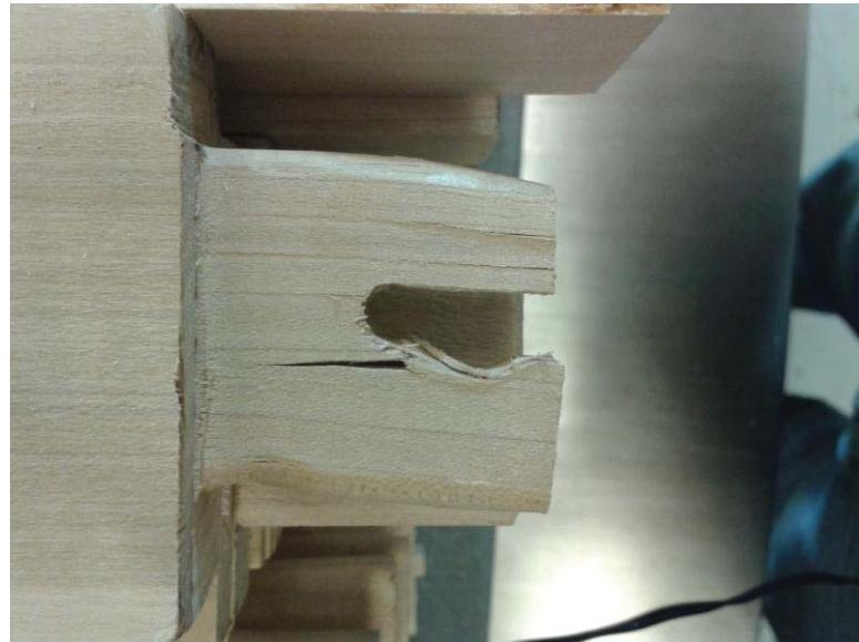
Failure on the stools with dowel joints.
