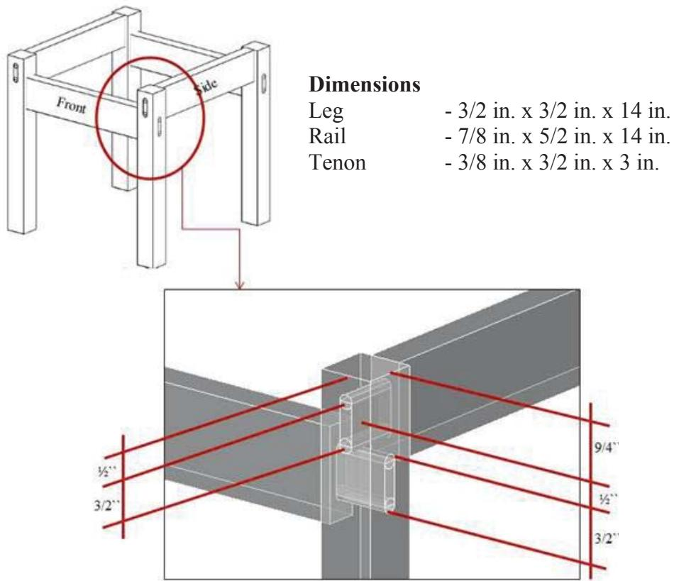
Figure 3-10: Glued round-shouldered rectangular mortise and tenon joint frame construction configuration.
