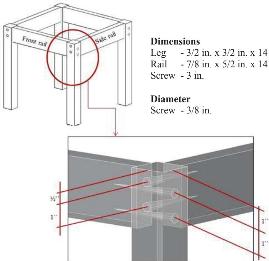
Figure 3-5: Screw joint frame construction configuration.
