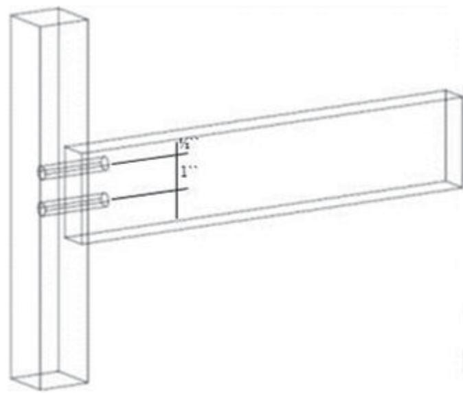
Figure 3-17: Dowel T-joint configuration.
