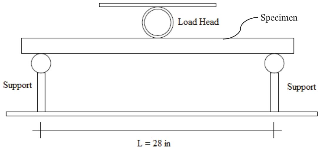
Figure 3-20: Test set up for determination of MOR and MOE.
