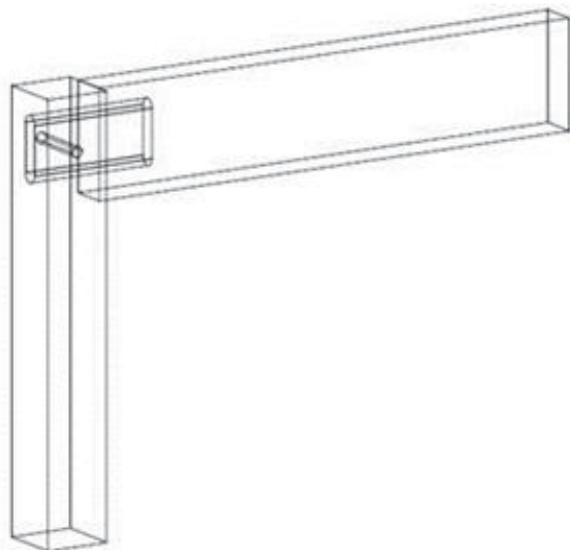
Figure 3-16: Pinned rectangle mortise and tenon L-joint configuration.
