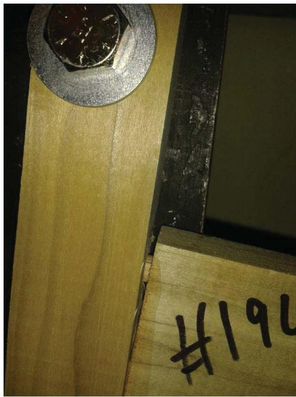
Failure on the T-shaped glued round mortise and tenon joints
