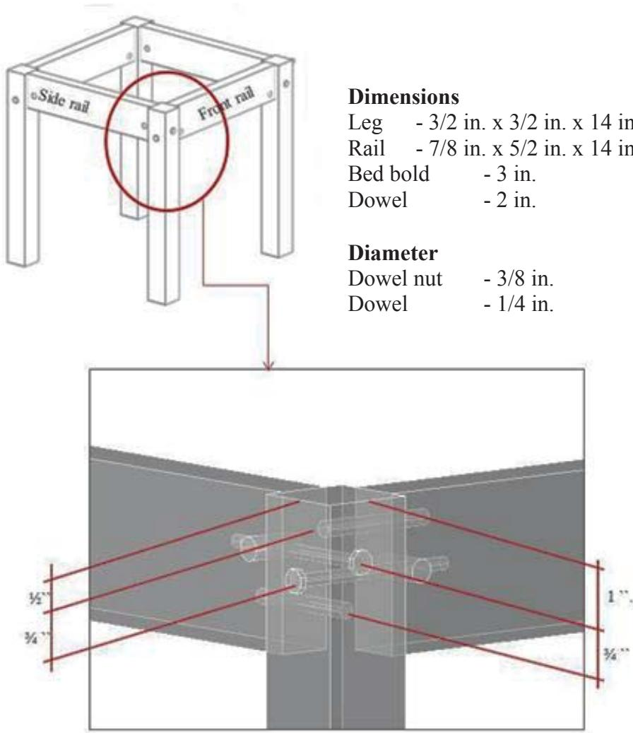
Figure 3-6: Bed bolt (Dowel nuts) joint frame construction configuration.
