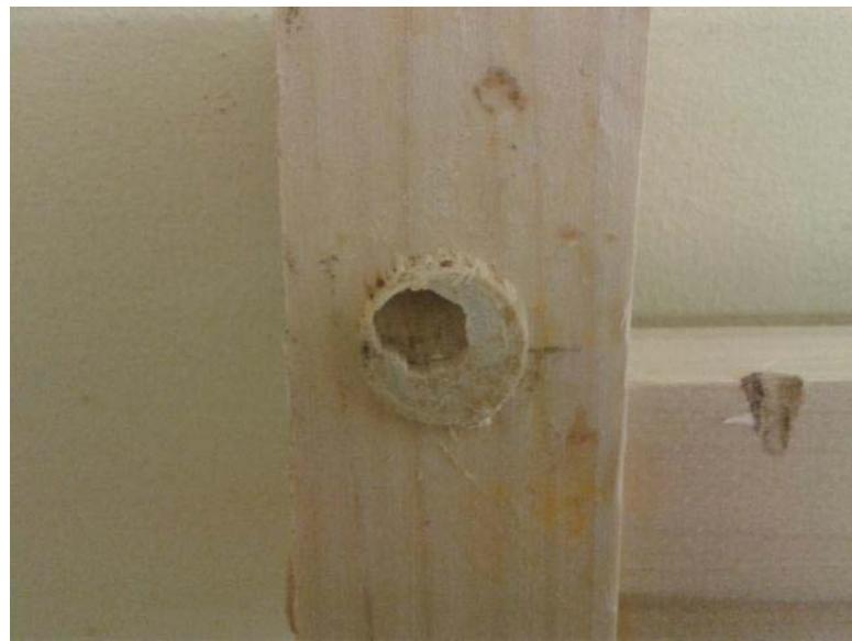
Failure on the stools with glued rectangular mortise and tenon joints.
