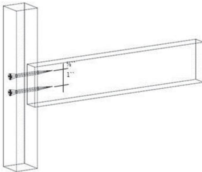
Figure 3-13: Screw T-joint configuration.
