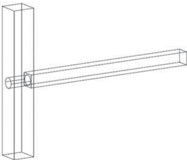
Figure 3-18: Glued round mortise and tenon T-joint configuration.
