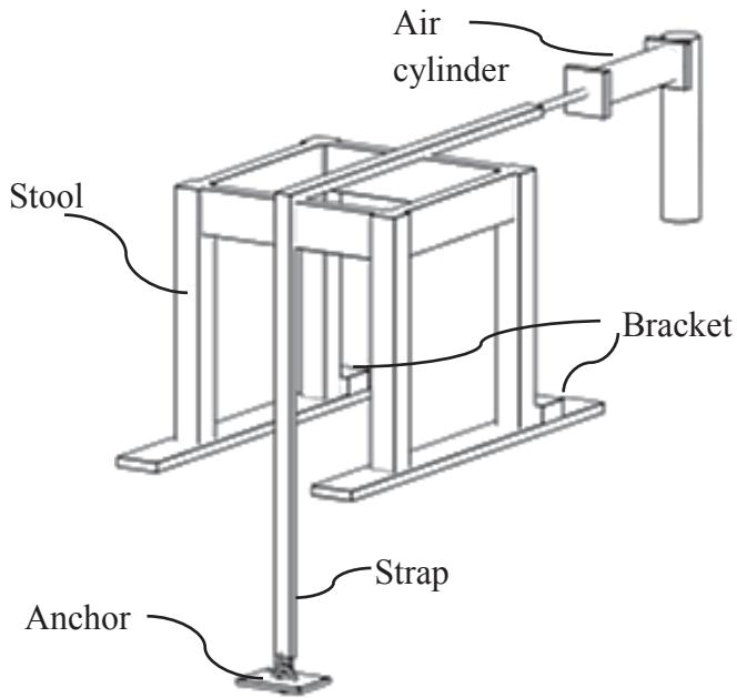
Figure 3-22: Cyclic front-to-back load test configuration.
