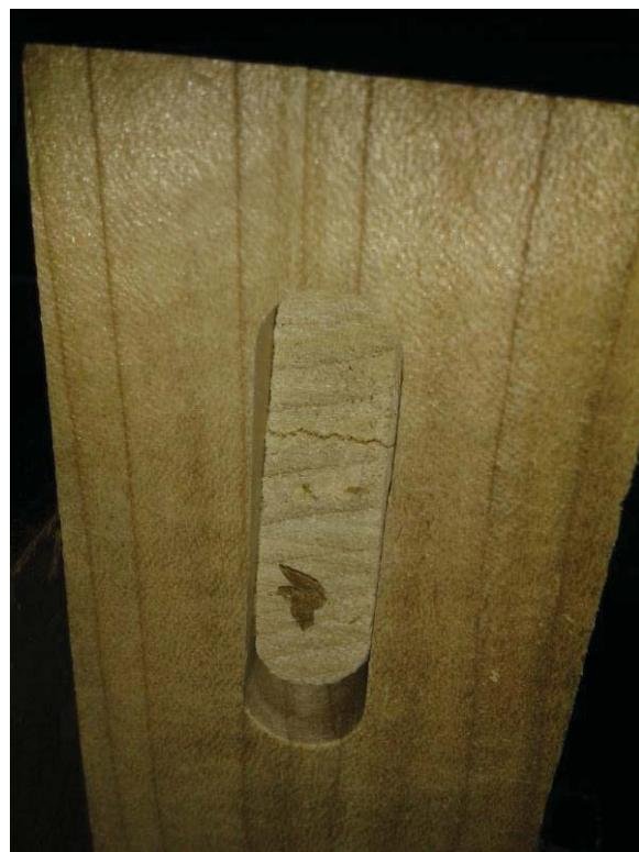
Failure on the T-shaped dowel joints
